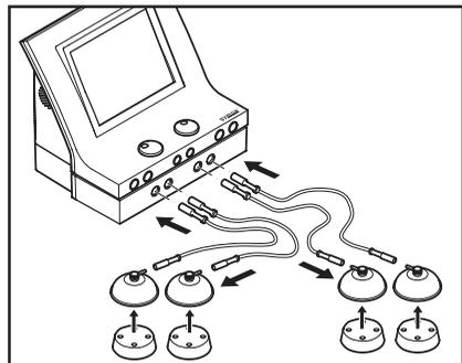
2. Connect the four vacuum hoses. Select two cables with the same hose colour for each channel.
