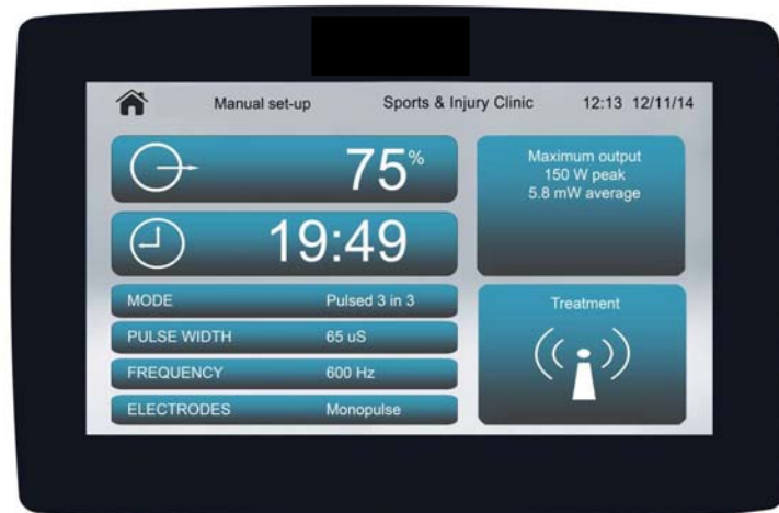
Fig. 22 Monopulse run screen
