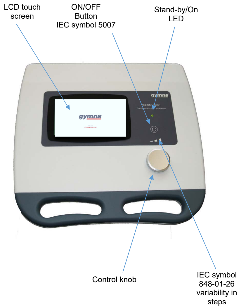
Fig. 3 Thermo 500+ control panel
