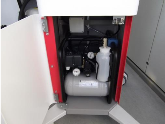
Fig. 7 Place the compressor into the trolley (as in the picture)
