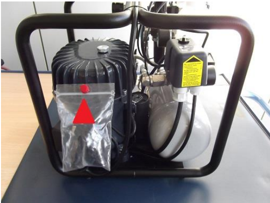
Fig. 1 Remove red cap (transport protection)
