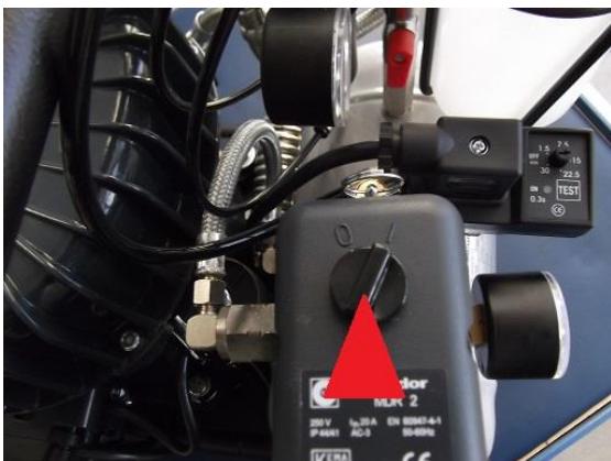
Fig. 5 Turn the start switch to position "1"
